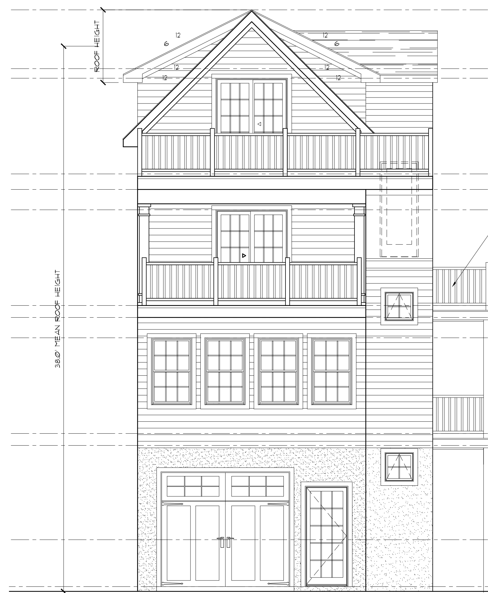
FRONT ELEVATION SCALE: 1/4" = 1'-0"
