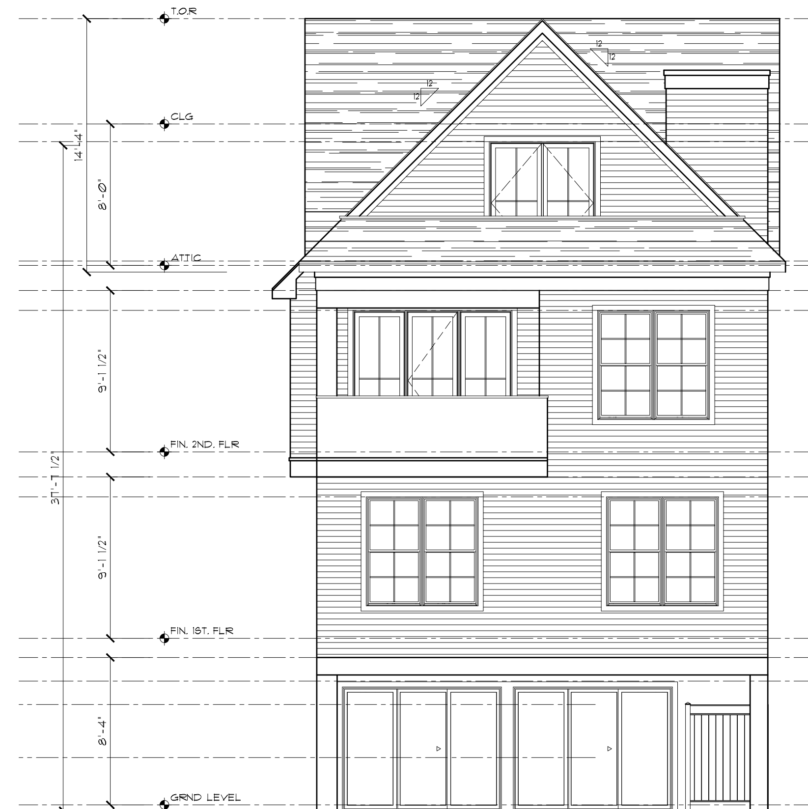
30 REAR ELEVATION SCALE: 3/16" = 1'-0"
