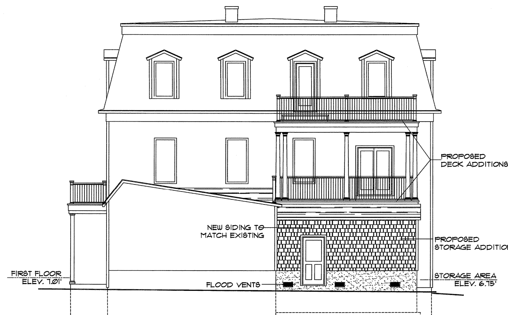
RIGHT SIDE ELEVATION SCALE: 1/4" = 1'-0" (EAST SURF STREET)
