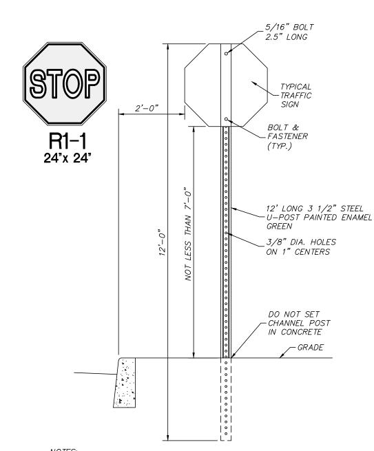
ALL REGULATORY & WARNING SIGNS SHALL BE HIGH INTENSITY REFLECTIVE SHEETING. ALL OTHER SIGNS SHALL BE ENGINEER GRADE SHEETING. ALL SIGNS AFFECTING COUNTY ROAD TRAFFIC SHALL CONFORM TO THE "MANUAL ON UNIFORM TRAFFIC CONTROL DEVICES", LATEST EDITION 4. SIGN POSTS SHALL BE 3LBS./FT..
