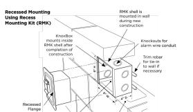
IMPORTANT: Care should be taken to ensure the front of the Recess Mounting Kit (RMK) shell housing, including the cover plate and screw heads, is flush with the wall. The RMK must be plumbed to ensure vertical
