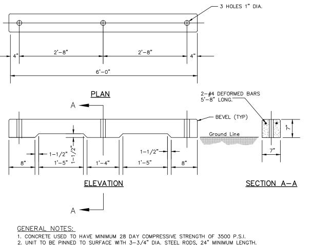
2. UNIT TO BE PINNED TO SURFACE WITH 3-3/4" DIA. STEEL RODS, 24" MINIMUM LENGTH. 3. ALL BEVELS TO BE 1/2". 4. ALL ANGLES TO BE 45.
