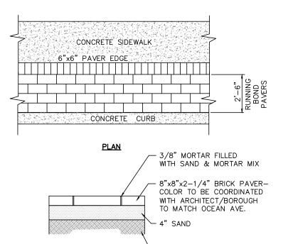
**BRICK SIDEWALK PAVER DETAIL** NOT TO SCALE
