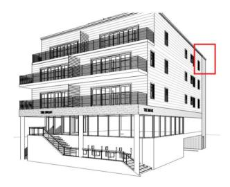
• Roof Decks & Terraces: Detail was added at the roof level - the stairwells no longer pop up to this level, the condensing unit farm is hidden at the rear corner of the roof, and
