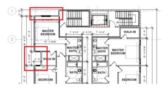
• **Stair Bulkhead:** We cut down the stairwell height to terminate at the same elevation as the roof.
