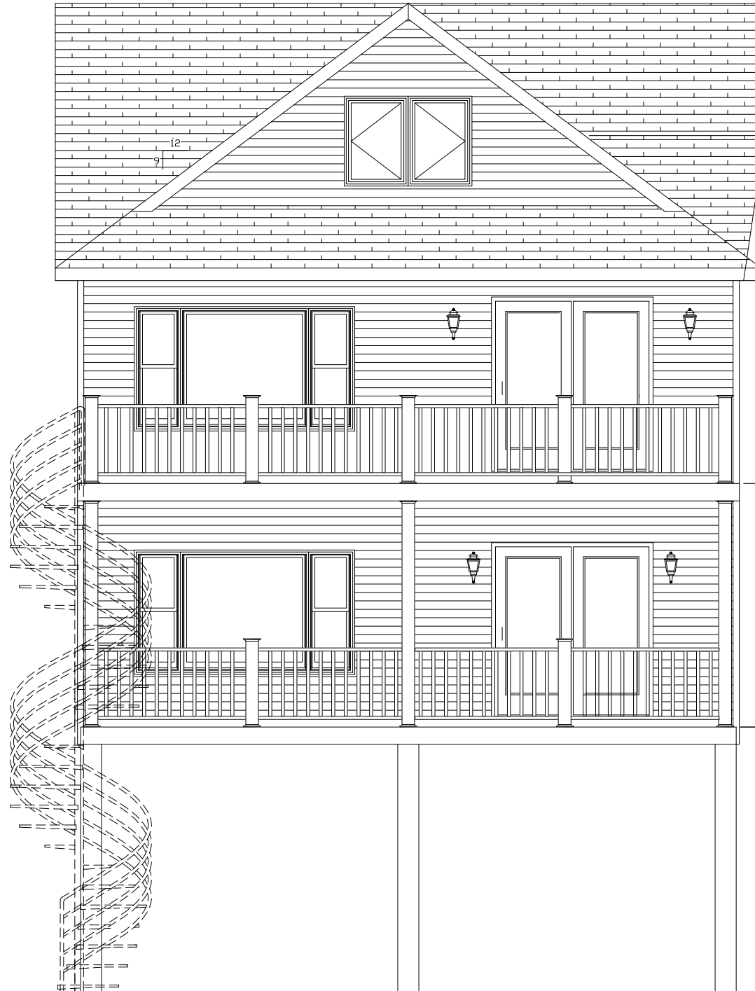
FRONT ELEVATION PORCH ROOF, DECK, STAIRS, RAILING, LANDING AND POSTS ON-SITE BY OTHERS
